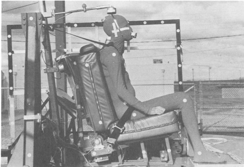
FIG. 2—Test subject clad and positioned on a standard seat. White disks are camera targets.
